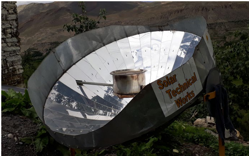
Figure 2: Solar cooker (picture by Solar Power Nepal e.V.; this society is dissolved by now)
